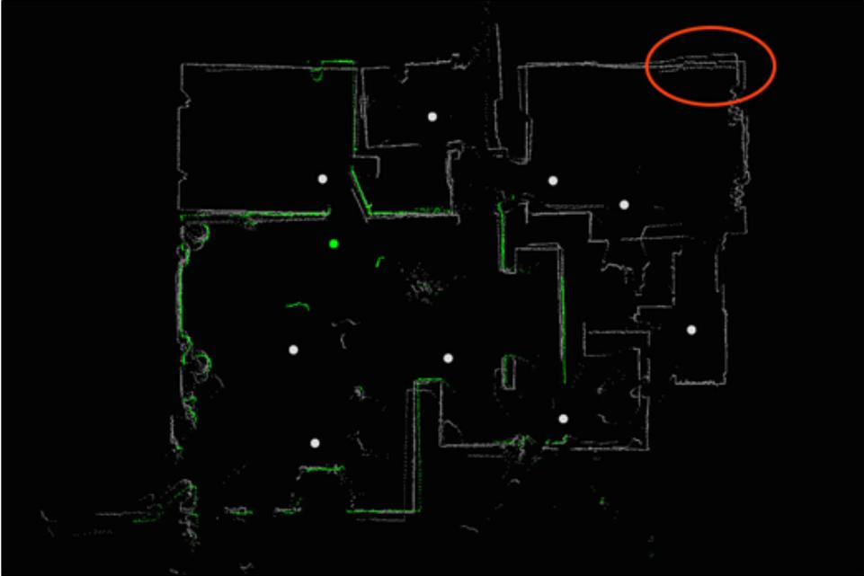
Figure 15. Not very well aligned data. Planitar drafting team may be able to correct room alignment, but will have to spend extra time doing that. Red-circled data resulted from improperly rotated camera. Reported dimensions for that room may be off.
