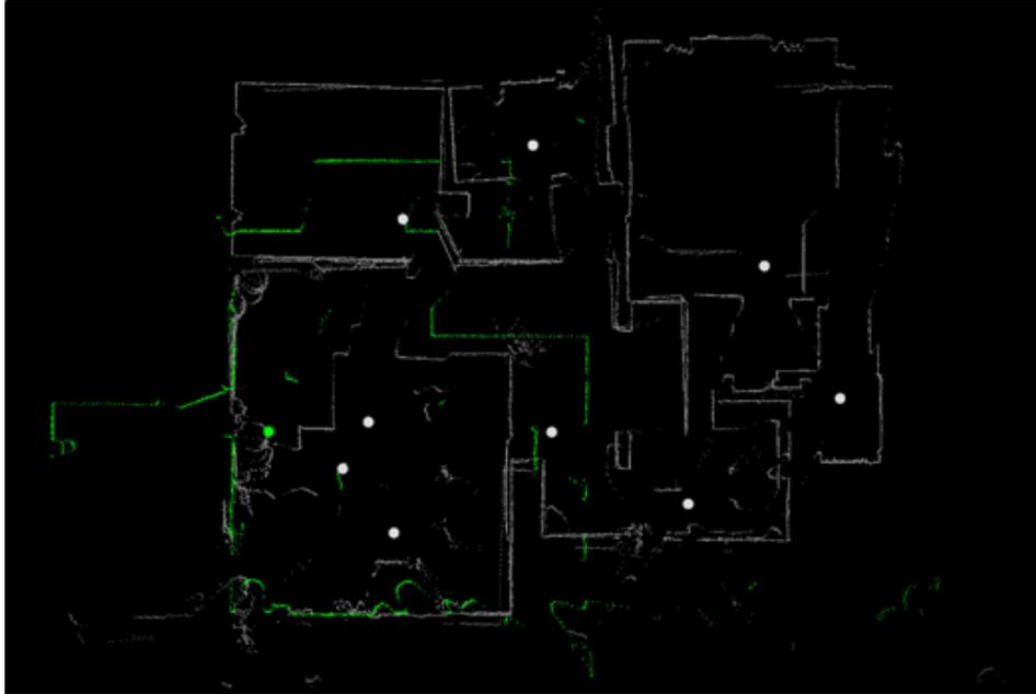
Figure 16. Badly positioned and aligned data. Planitar drafting team will not accept this data for drafting until all rooms are positioned on the floor in the correct relationship and are sufficiently aligned.
