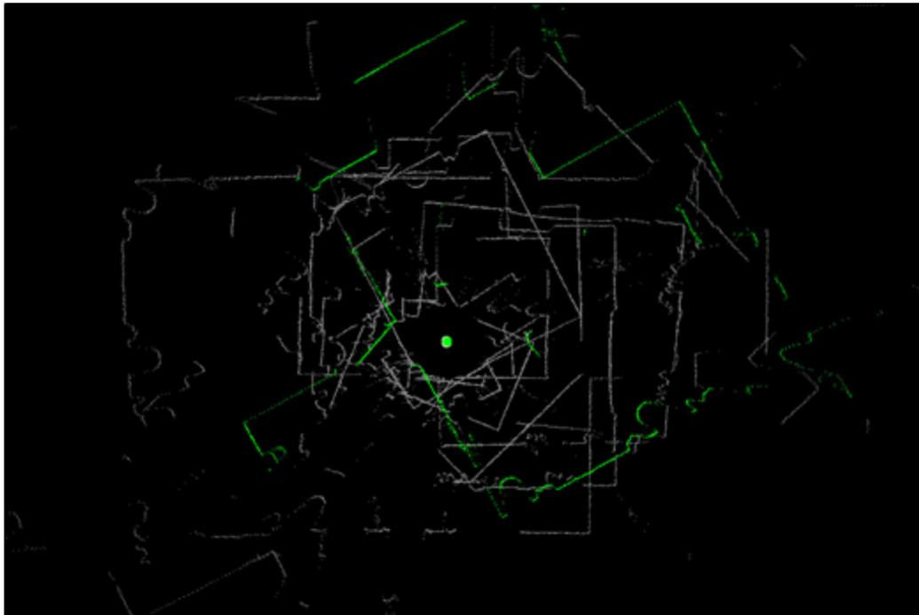
Figure 17. Completely unaligned data. Planitar drafting team will not accept this data for drafting until all panoramas are properly positioned and aligned.
