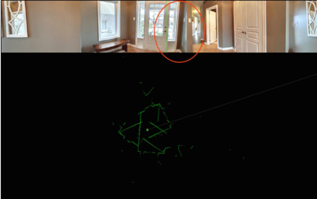
Figure 18. Wrong panorama rotation direction. It must be corrected in Stitch by using the Reverse Camera Rotation option.
