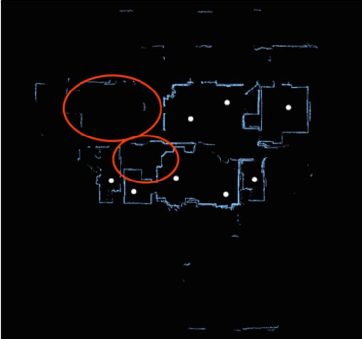
Figure 19. Missing room data - not all rooms on the floor have image data, so windows and other features cannot be shown properly on the floor plan. Planitar drafting team will not accept this data for drafting.
