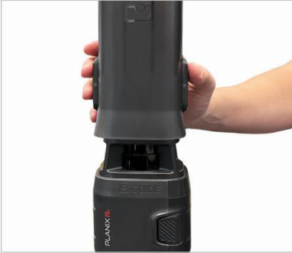
Remove the system shield by pressing on the release tabs and pulling the system shield up while holding firmly onto the PLANIX R1's base.
